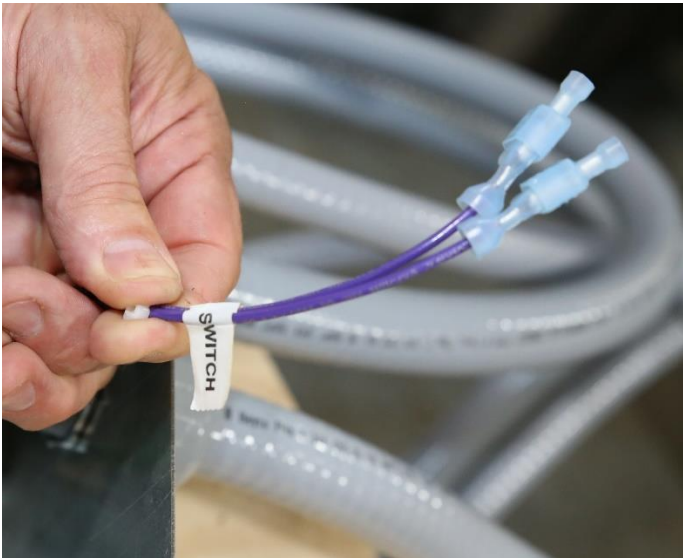
Door Switch wires are purple and are labeled, if There are 2 door switches, wire door switches in series.
